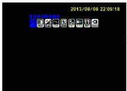
Pressing the center key opens the on screen menu top level, as shown in the picture to the left.
