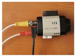
Connect the BNC video cable to the camera and the other end to your monitor or video capture device.
