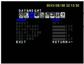
The camera must be set to DAY if you want to observe in color. The camera must be set to NIGHT if no color (B&W only) operation is desired.
