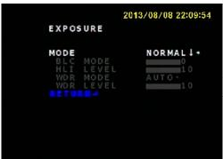
**NOTE:** Normal mode is linear. HLI, BLC, WDR are NOT linear and stretch the histogram based on different curves
