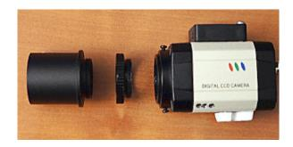
The camera has a standard CS-mount with a mount flange to sensor 12.5mm distance. If this distance is too small, it can be increased by adding spacers. Your camera was shipped with 1 pc. 5mm C-mount spacer.
