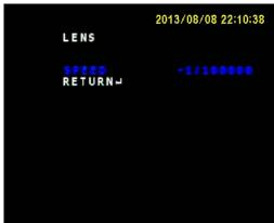
Once in the ELECTRIC sub-submenu, scroll left and right to find the exposure time you need. Available values are from the longest single frame integration of x1024 cycles (17sec) to the shortest value of 1/100,000 sec (that is 10 microseconds).
