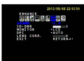
The GAMMA setting can be adjusted from 0.3 to 1.0. A value of 0.3 brings up the most details from the dark image areas but a value of 1.0 has the most contrast. A value of 1.0 is used with LCD.
