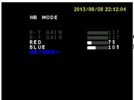
In manual mode you adjust the gain for the colors RED and BLUE. A good starting point are the values shown in the left image.
