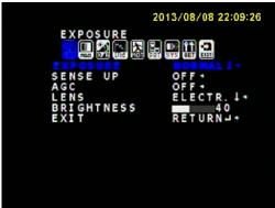
Press the center key again and it opens the submenu for the icon that was highlighted in blue.
