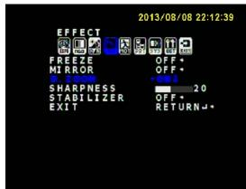
Under the EFFECT menu you can FREEZE/UNFREEZE the image but this function is performed a lot simpler by using the remote.
