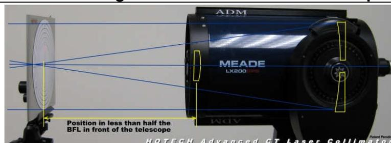
The distance between the laser collimator and your telescope varies depending on the diameter and focal length of your telescope. In general, the greater the distance from the telescope, the higher accuracy you will achieve. In practice, any distance beyond the focal distance will be sufficient. In this procedure, we will identify the best collimating distance for the telescope.
